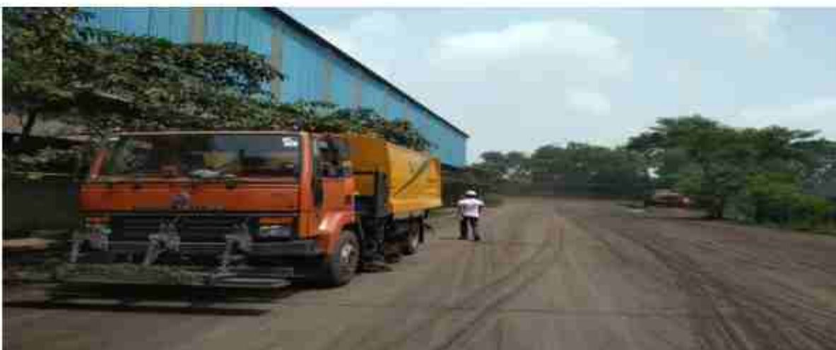
Road sweeping machine to control fugitive dust from road during transportation
