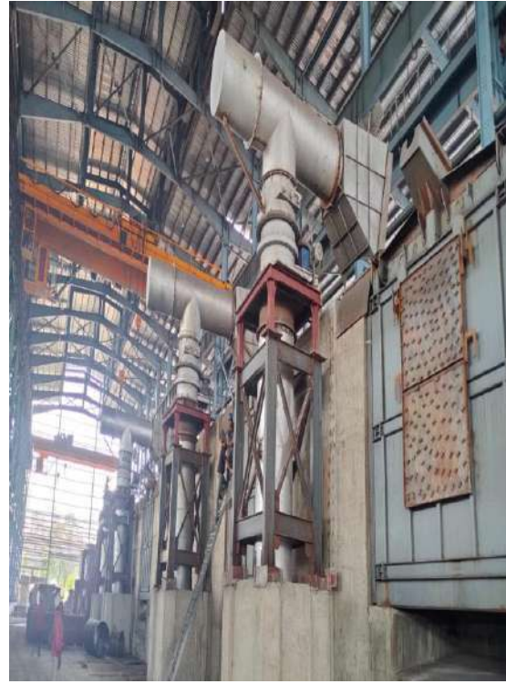
Induction furnace connected with primary hood
