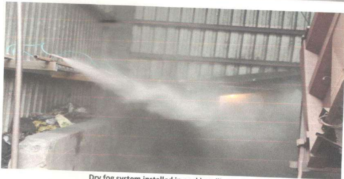
Dry fog system installed in coal handling system
